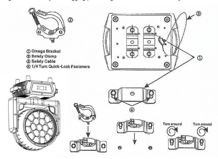
Regardless of the rigging option you choose for our fixture, always be sure to secure your fixture with a safety cable. The fixture provides a built-in rigging point for a safety cable on the hanging bracket as illustrated above. Be sure to only use the designated rigging point for the safety cable and never secure a safety cable to a carrying handle.
